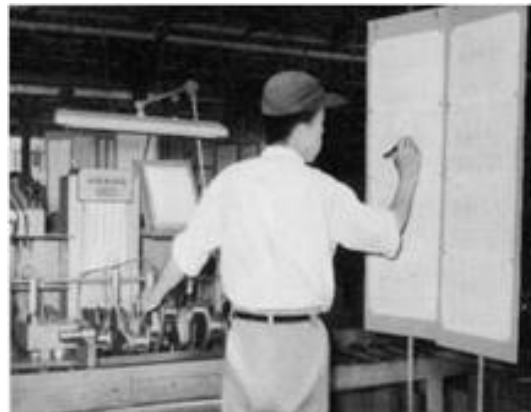
Figure 9: Writing Fishbone Chart at a Toyota factory for identifying causes of defects
