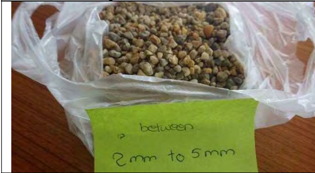
Sample of filtration gravel, 31 March 2017
