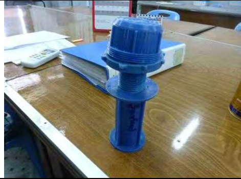
Strainer of Existing WTP, 02 May 2014
