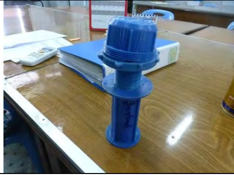
Strainer of Existing WTP, 02 May 2014
