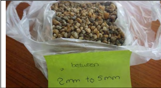
Sample of filtration gravel, 31 March 2017
