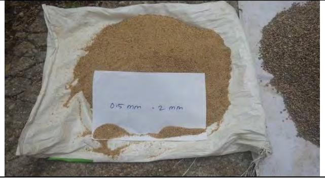
Sample of filtration sand, 13 Oct. 2016
