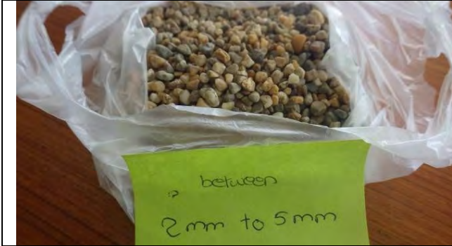
Sample of filtration gravel, 31 March 2017
