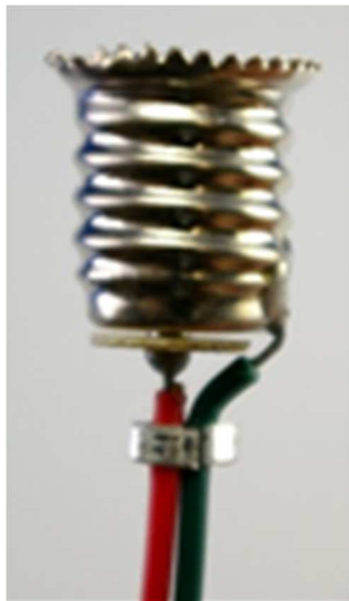
Photo when the plastic cover of the miniature bulb holder is removed
