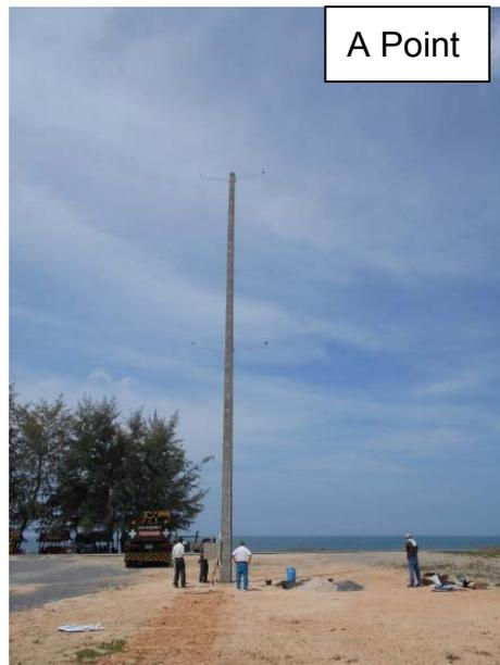
[High pole for Wind Measuring Device : A point]
