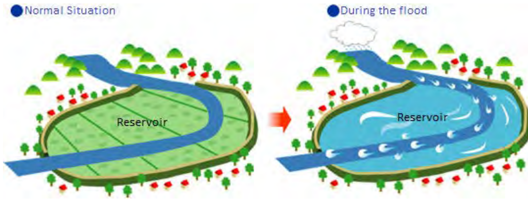
Figure Summary of the function of flood control with reservoir (Source: Iwate Office of the river and national roads, Ministry of Land, Infrastructure, Transport and Tourism, Japan (MLIT))
