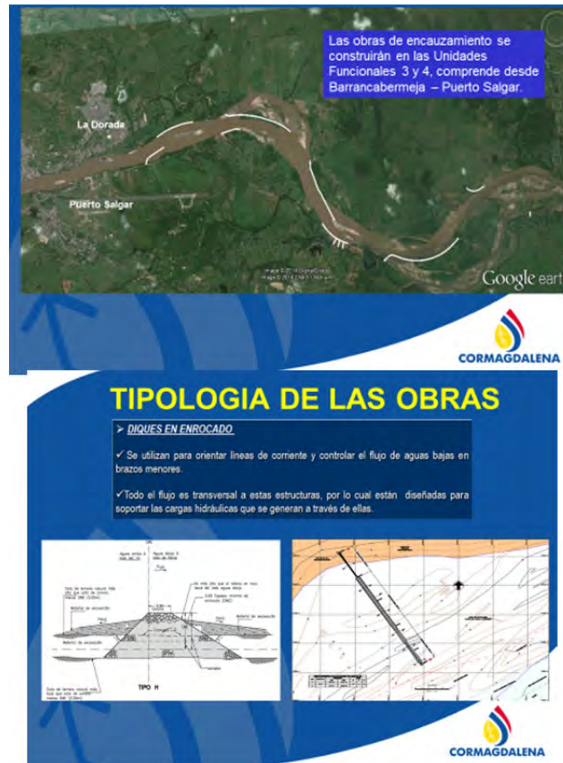
Figure 6.3 Submerged Dikes to Maintain the Navigable Channel
