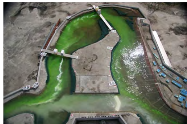
Figure 7.8 Examples of Experiments with a Water Channel Model (left: full model, right: example of channel rectification)
