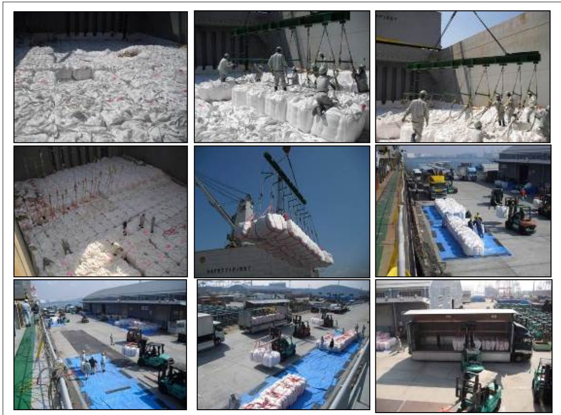
Figure 5.2.4-3 Handling method with big bags
