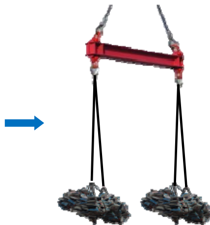
Figure 5.2.4-2 Handling method by Lifting beam equipped with 2 hooks
