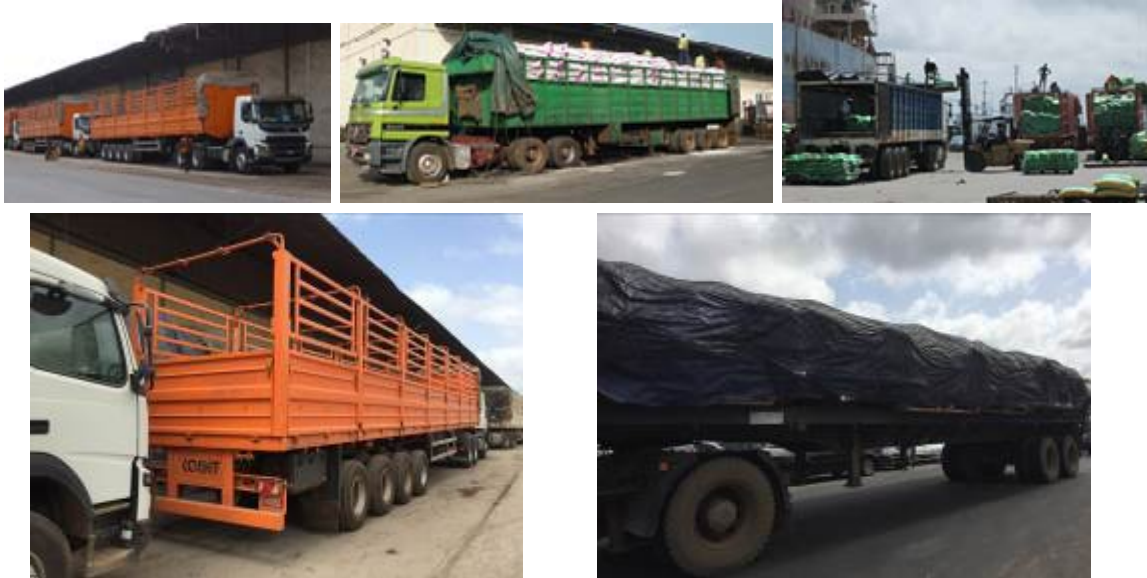
Overall length 18.5 m, vehicles with side walls, 4 axis vehicles (65 ton loading vehicle) Vehicles with awning sheets on loading pallet products
