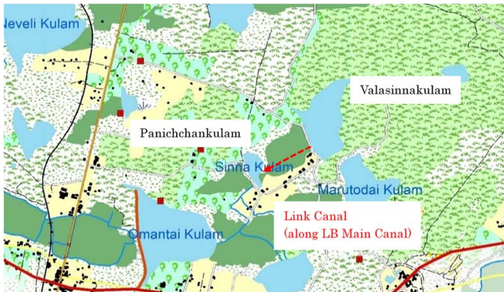
Figure 7.2.2 Schematic Layout of Link Canal in Naveli kulam Cascade System
