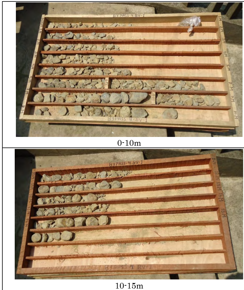
Figure 2-2 Core Photos (BV-1)
