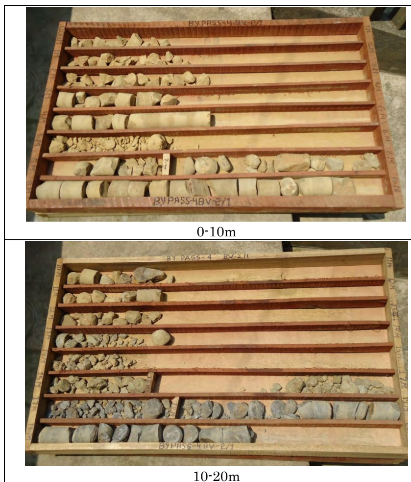
Figure 2-3 Core Photos (BV-2)
