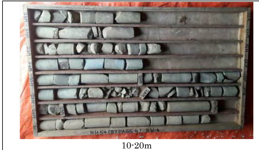
Figure 2-6 Core Photos (BV-4)
