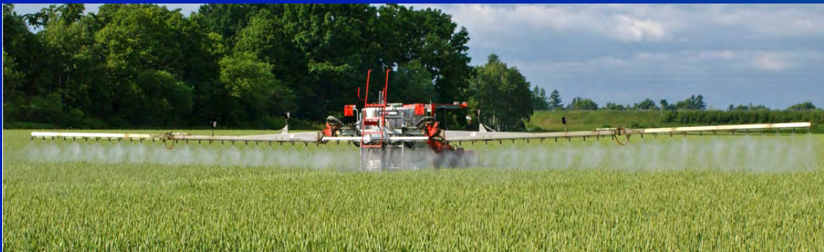
Tractor mount type (both side boom) (1500L 18m)
