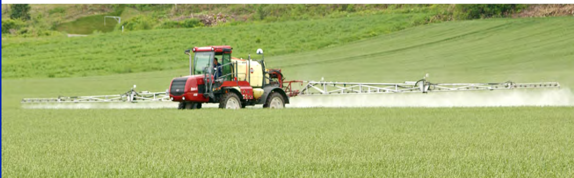
Self propelled type (5000L 31m)
