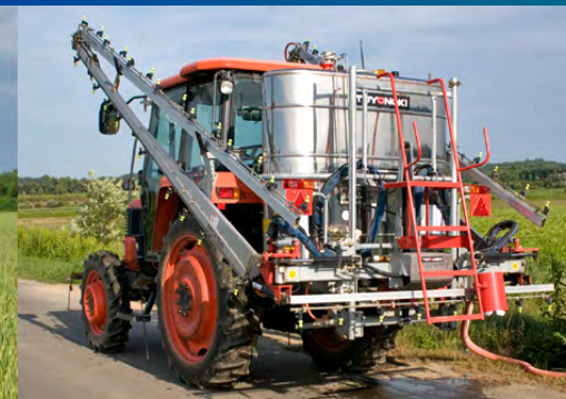
Tractor mount type (both side boom) (1500L 18m)
