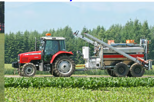
Tractor mount type (both side boom) (1500L 18m)
