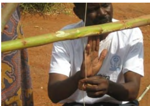
16) Tiyeze utali wa chingwe kuchokera pa mtengopo kifika pamene tingamangirire mwala pogwiritsa ntchito dzanja ndipo tiyikepo chizindikiro.
