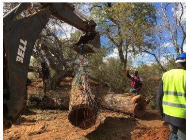
d. Measuring the total fresh weight of each part (measuring for the stem in the photo)
