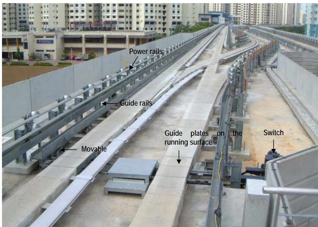
Figure 2-37 Appearance of the Track Course (running surface, guide rails, switches)
