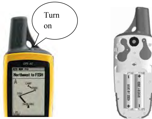
Figure 7.2. Turning on GPS and Installation of Batteries
