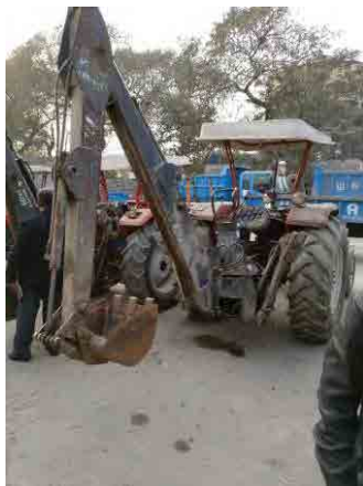
Koyker Backhoe with regular bucket
