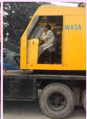
Broken door & No seat belt
