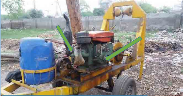
Non-Functional Bucket Machine (Winch Machine)
