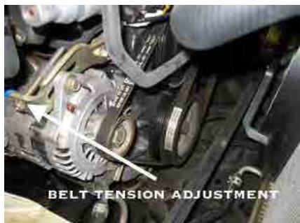
Fig. 1: A gauge is recommended, but you can check belt tension with thumb pressure
