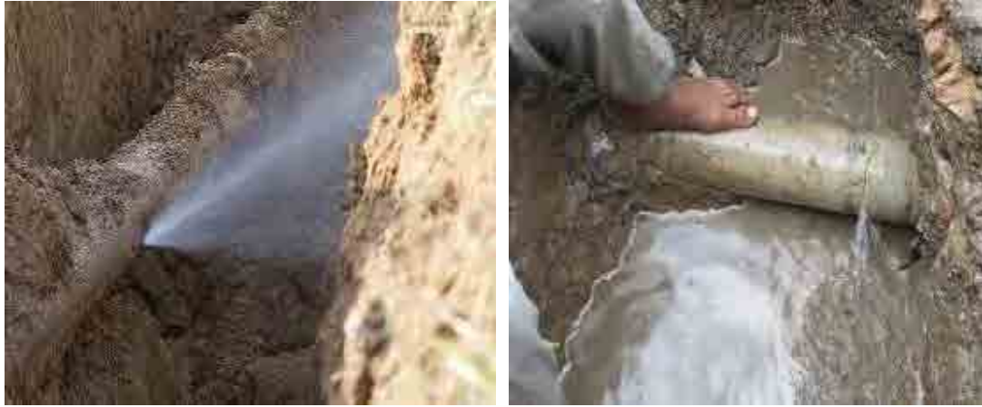
Figure 1: Water Loss from hole (left) and crack (right) of an Asbestos Cement Pipe
