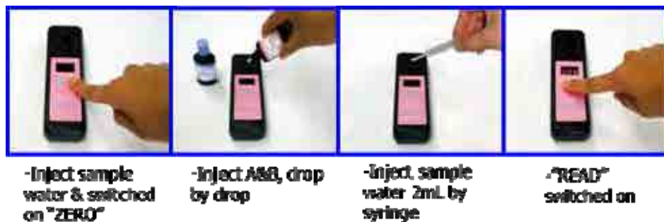
Figure 11: Leak Detection by Residual Chlorine Detection
