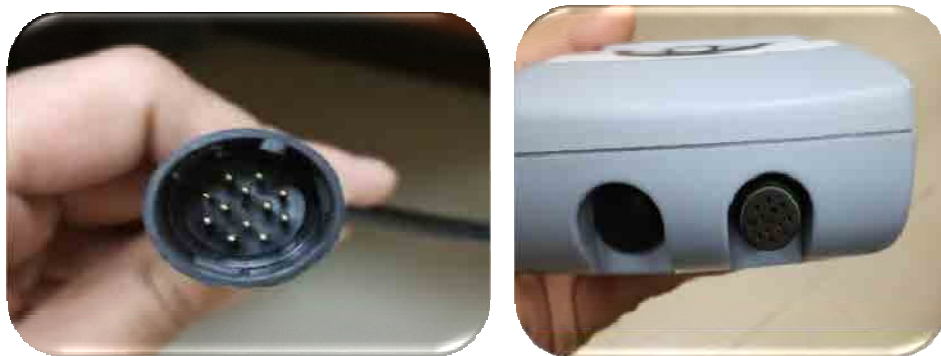
Figure 21: Plug connection with ultrasonic meter
