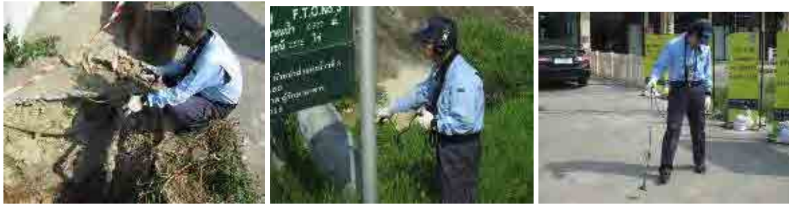
Figure 6: Acoustic Survey with Leak Detector
