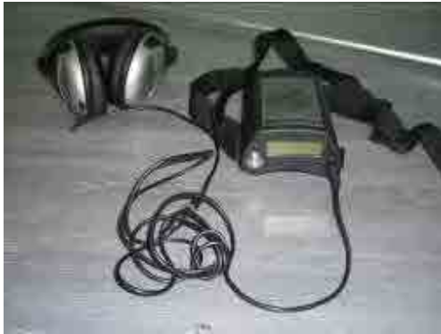
Figure 4: Headphone Attached with Amplifier (Left) and Hand Probe Microphone (Right)
