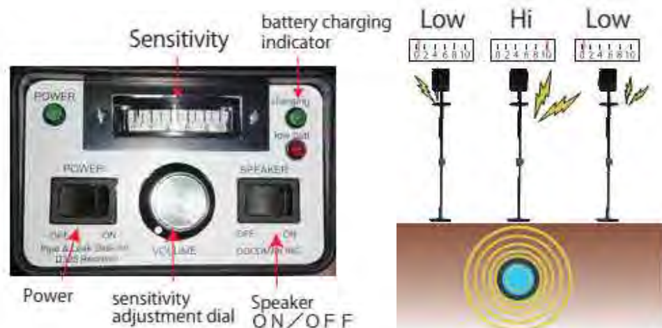
Figure 5: Antenna Sensitivity Adjustment with Movement
