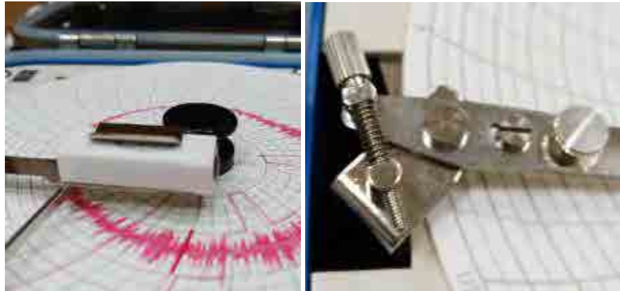
Figure 14: Cartridge Pen Adjustment
