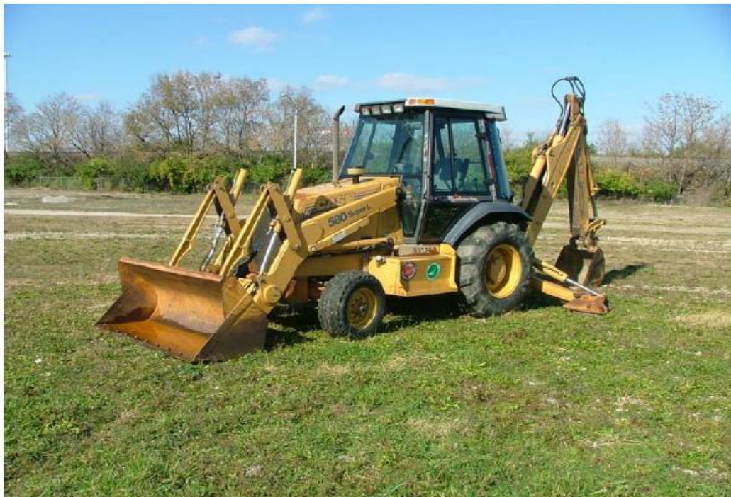
Figure 6: Backhoe with a front load
