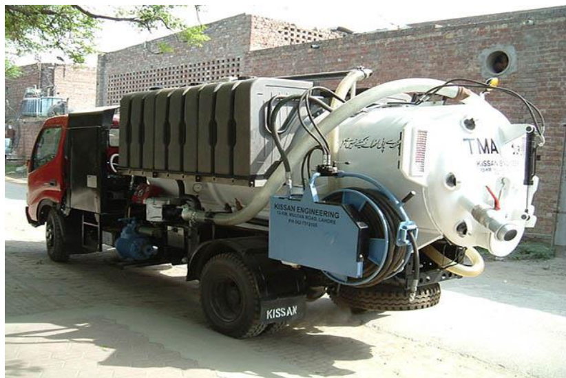
Figure 11: Combined Unit (suction off PTO Jetting with axillary pump 150 to 200 bar)
