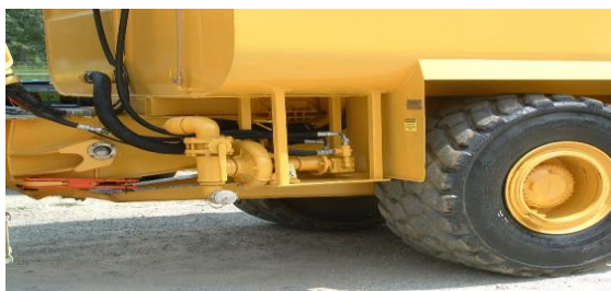
Figure 16: Water Tanker Centrifugal Pumps (PTO and stand-alone engine driven)
