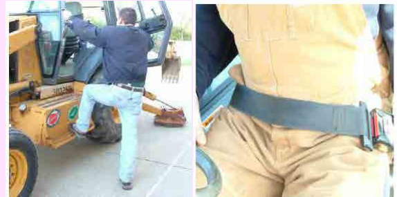
Proper Mounting with three point contact and wear a seat belt
