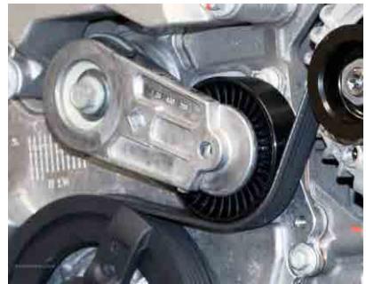
Fig. 1: A gauge is recommended, but you can check belt tension with thumb pressure
