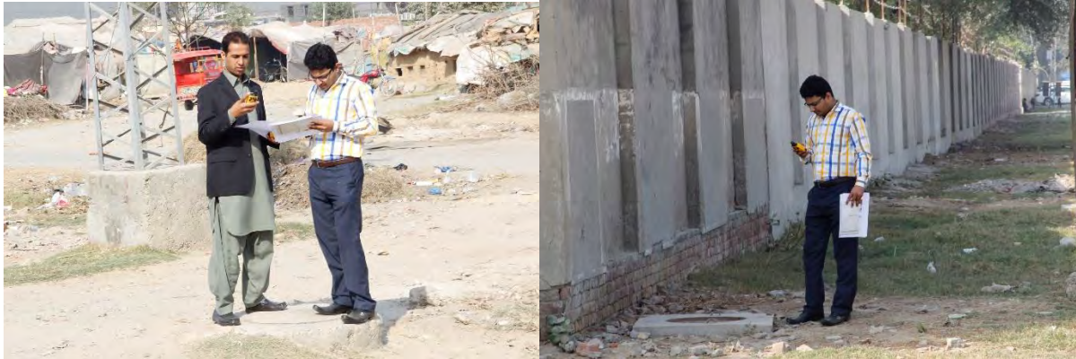
Figure 24: Marking Location of Manhole by Using GPS
