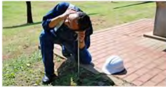
Figure 2: Use of Acoustic Rod
