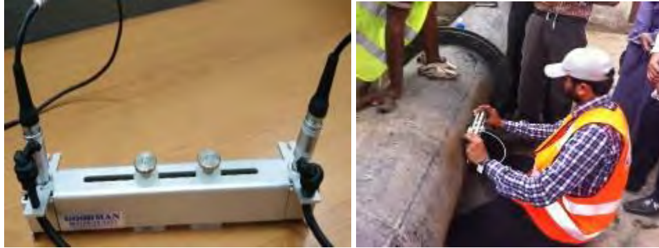
Figure 17: SE 1586 Probe Installation
