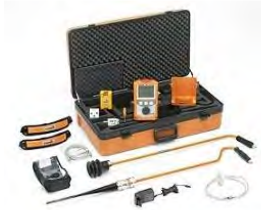
Figure 4: Tracer Gas Sampling Equipment (source: Sewerin Technologies)
