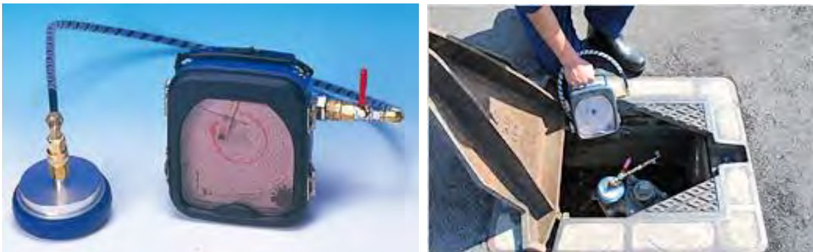
Figure 9 (a): Working of Pressure Recorder
