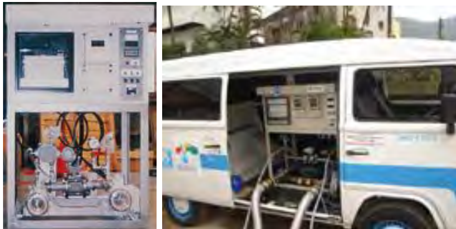
Figure 6: Pictorial View of Mobile Type Electromagnetic Flowmeter (Source: FUJI TECOM INC. and JICA Project in Brazil)
