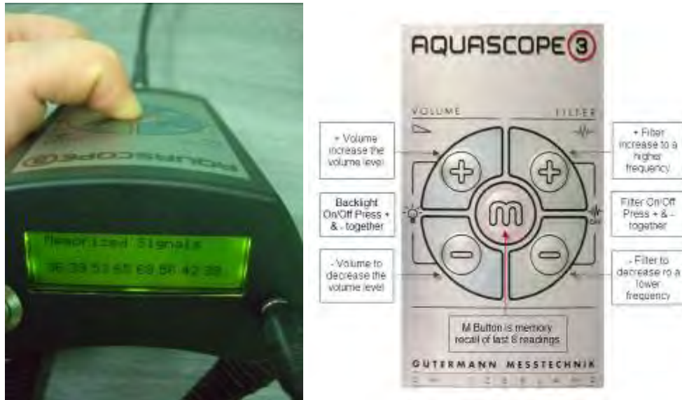
Figure 9: Memory Data (Left) and Labeled Buttons on Amplifier (right)
