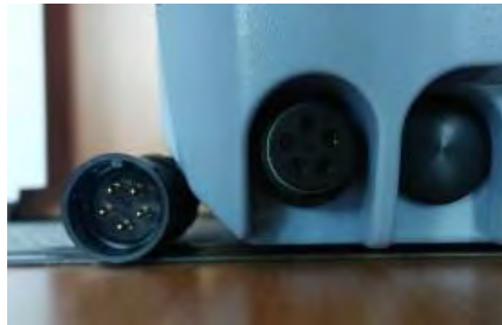
Figure 18: Probes Wires Connection
