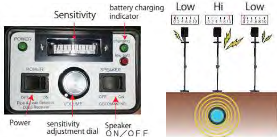
Figure 5: Antenna Sensitivity Adjustment with Movement
