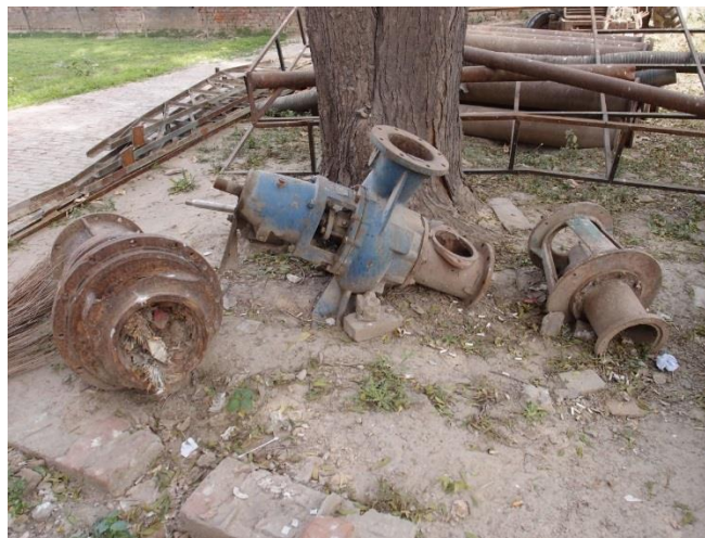
Plate 2: Improper Storage of Damaged Valves and Pipes in Stock Yard
