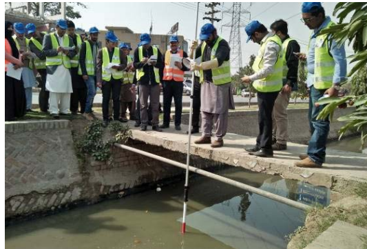
Photo 10: Field activity of measuring sludge volume
