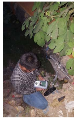
Picture 6.9 Installation and Measurement of Flowrate by Ultrasonic Flow Meter on June 8, 2017
