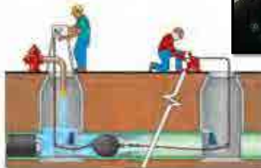
3. Introduce water into manhole and slowly release Ball down the line.
