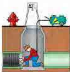
1. Install Plug to isolate manhole.
