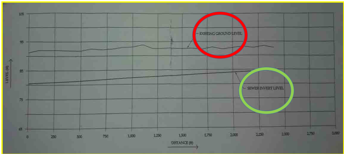
Profile of Sewer Line
