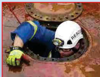
Manhole – A Confined Space
