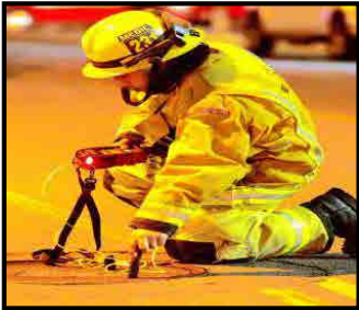
Gas Monitoring at Manhole
