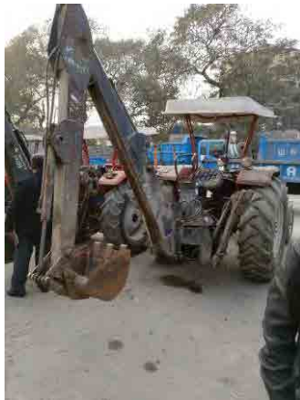
Koyker Backhoe with regular bucket
