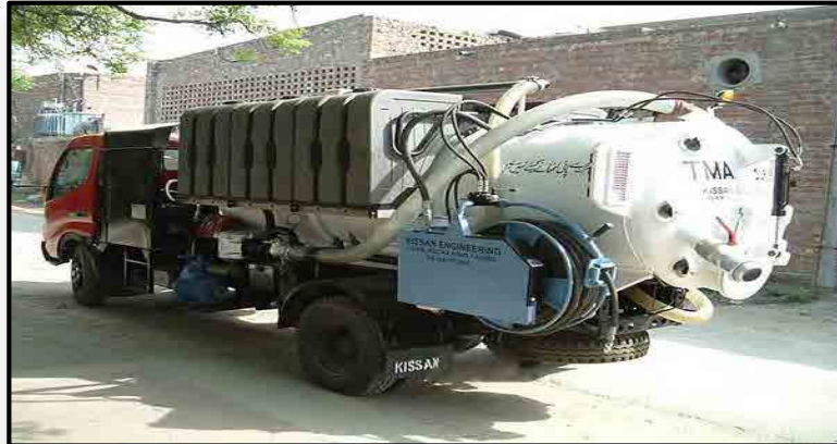
Combined Unit (suction off PTO, Jetting with axillary pump 150 to 200 bar)
