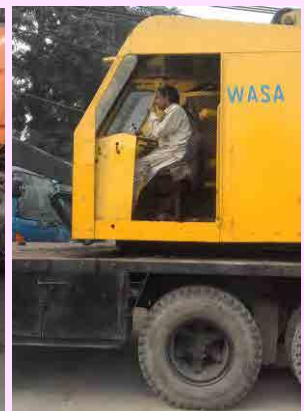
Broken door & No seat belt
