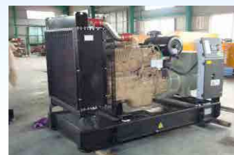
Main frame of Diesel Generator
