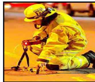
Gas Monitoring at Manhole
