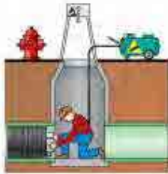
1. Install Plug to isolate manhole.
