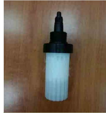
Check the Clogging in filter
