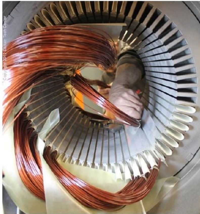
Figure 5 Stator re-winding for Induction motor
