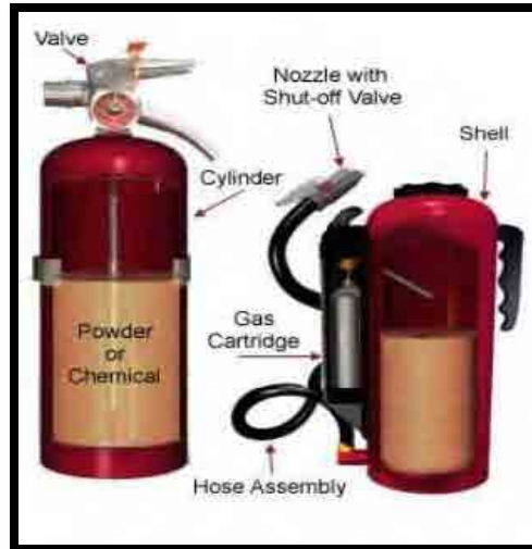
Figure 9: Portable Fire Extinguisher
