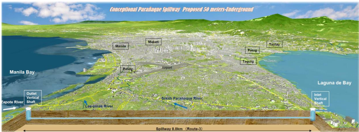
Figure 8.1.2 3-Dimensional Image of Parañaque Spillway
