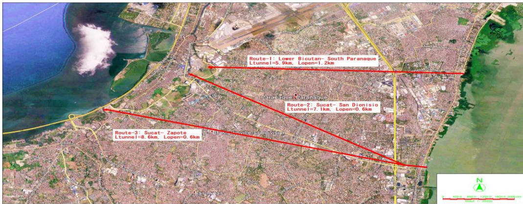
Figure 8.1.1 Alignment Alternatives of Parañaque Spillway
