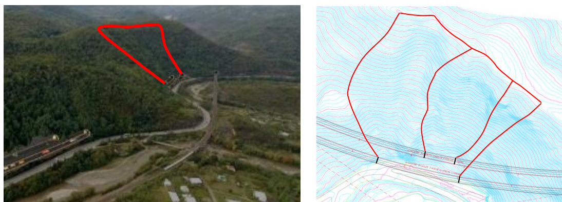
Figure 4-68: Range of Rockfall Sources Reaching the Road
