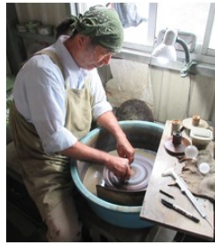
Uses a Large Disk. A stone is held by hand.
