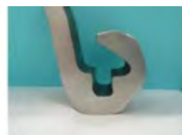
Expandable water cut-off material (water expandable rubber, silicon, bentonite, etc.)
