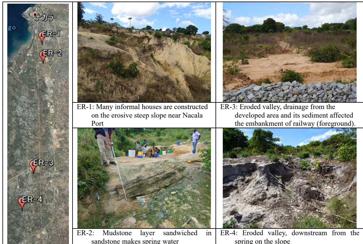
Figure 3.1.5 Example of eroded slope on the Cretaceous sandstone (CtMo) layer
