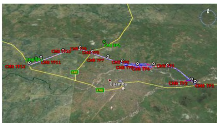
Figure 8.2.13 Location of Soil Sampling for Existing Ground and Borrow pits (Cuamba Bypass Road)
