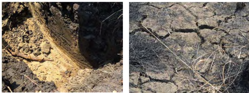
Figure 8.2.14 Ground Surface Covered with Thin Organic Soil and its Particular Cracking
