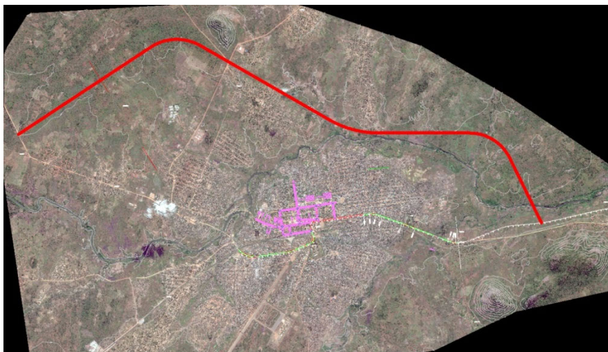
Figure 7.7 Selected Route/Alignment of Cuamba Bypass Road
