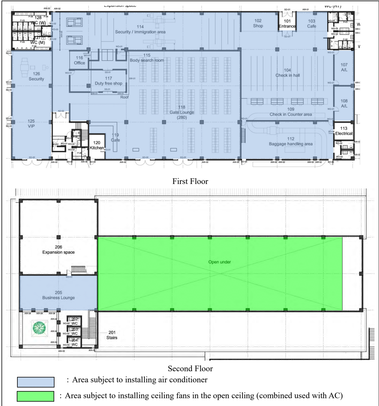
Figure 27 Areas Subject to Air Conditioning (IDT)
