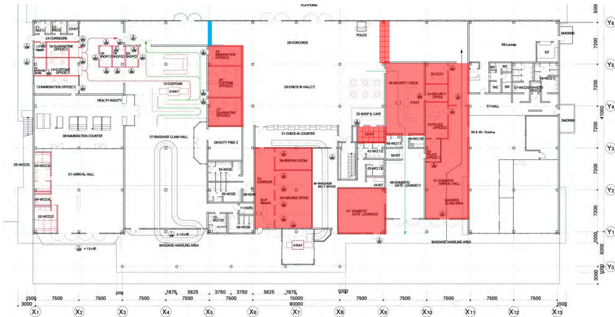
Figure 88 ETB Rehabilitation Sequence (Phase 2)
