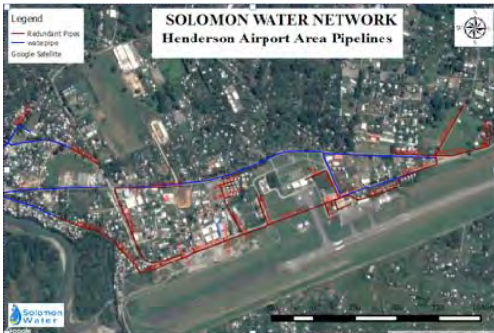
Figure 26 Water pipe Network around the Airport
