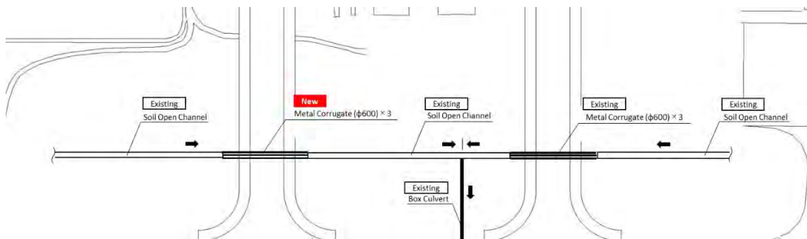
Figure 36 Taxiway Drainage Layout
