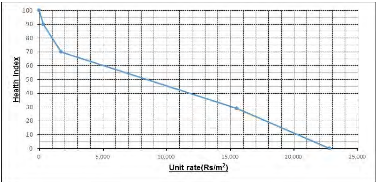
Figure 3.1.2.1 Relation between HI and unit rate
