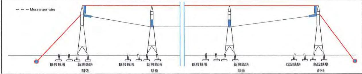
Step-21 Set stay wire at the strung conductor and proceed the same for the adjacent string span Shut down
