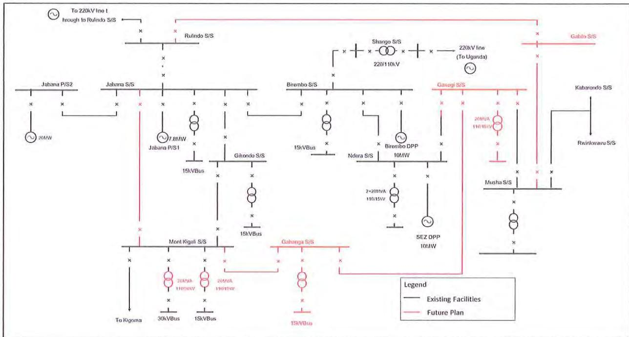
Figure 2.6-1 Range for power flow analysis
