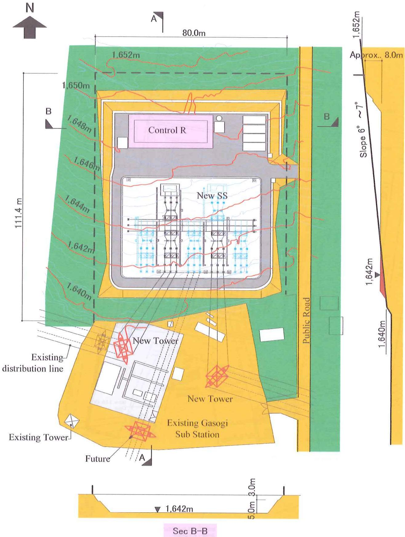
**New Gasogi Sub Station Layout plan**
