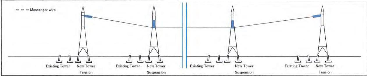
Step-20 Set stay wire to the position of strung conductor and proceed the same for next conductor Shut down
