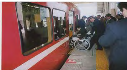
Equipment to eliminate steps and gaps, stored at a platform of Kami-Ooka Station on the Keikyu Main Line.
