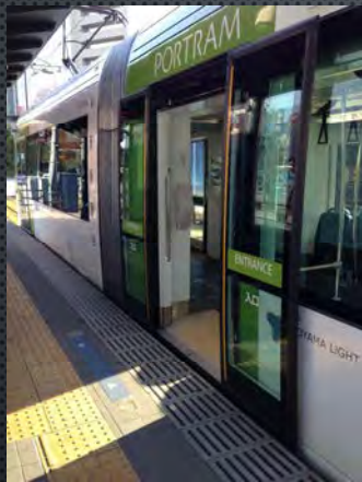
5mm gap height is realized. (in Toyama LRT)
