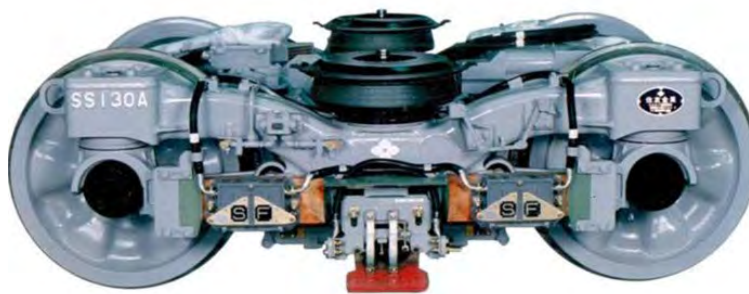
Figure 4.6.4 Sample of Bolsterless Bogie with 3rd Rail Collector
