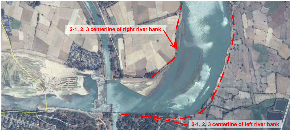
Figure 2-2: Location of Center line profile survey & longitudinal cross section survey along the river dike
