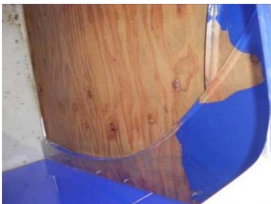
Tank H : Corruption of tank back board
