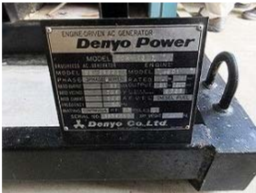
Nameplate of generator set
