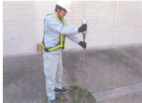
1-2b Cone Penetration Test
