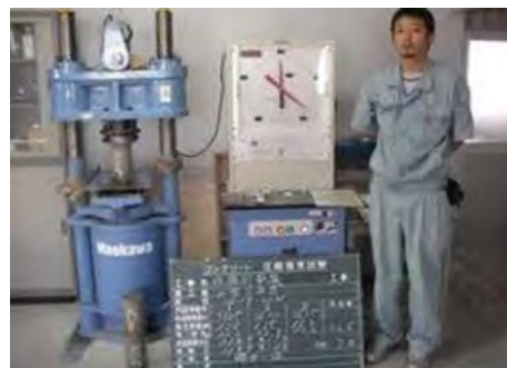
1-10b Concrete compression test
