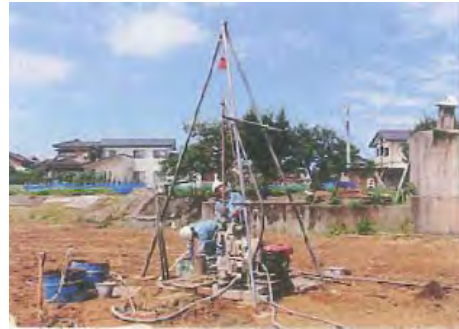
1-2a Standard Penetration Test
