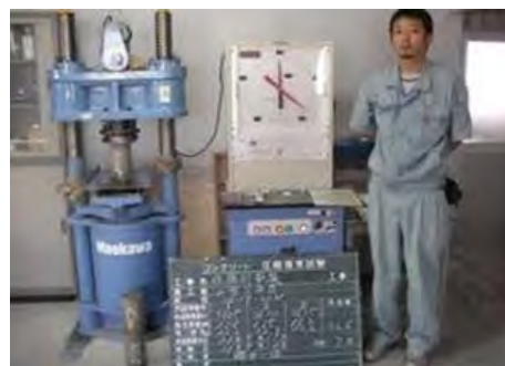
1-10b Concrete compression test
