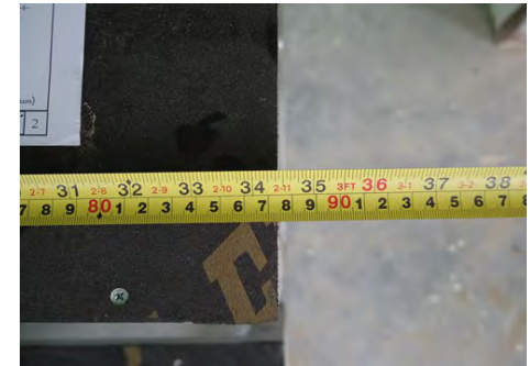
4-13b Size was smaller than drawing
