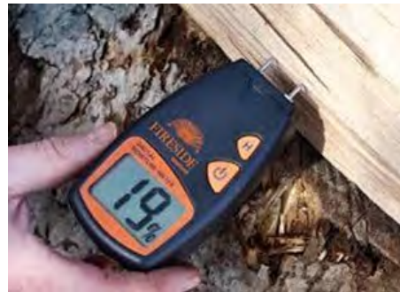
3-3a Check water content before installation
