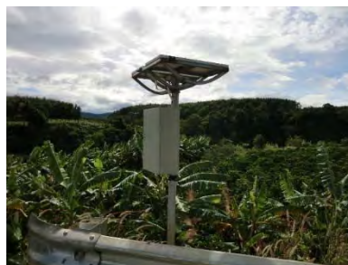
Fig 8. Telemetric river water level gauge installed by International University of Ho Chi Minh at Dak Pxi river in Aug. 2017.
