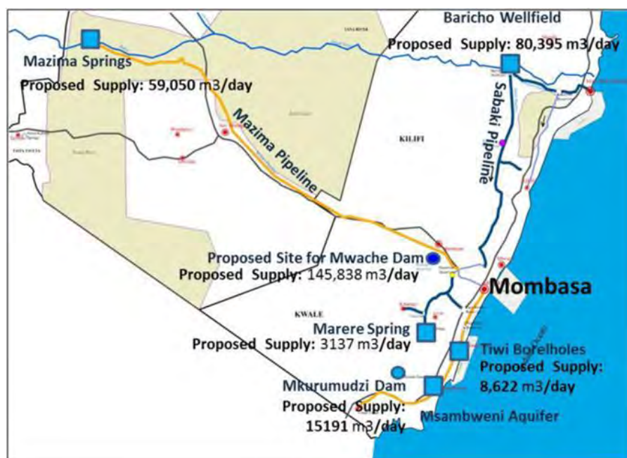
Source: ISUDP for Mombasa Town as KMP (Draft ISUDP Proposals Report, August 2015) Figure 5.1.8: Water Supply Trunk Infrastructures for Mombasa County
