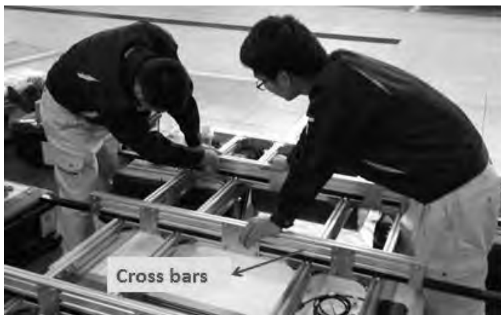
Figure 12.12 Attach the cross bars to platform
