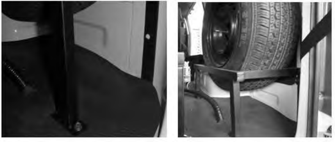
Figure 12.22 Fix the spare wheel to its frame
