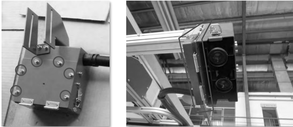
Figure 13.6 Where to Remove the Camera Case
