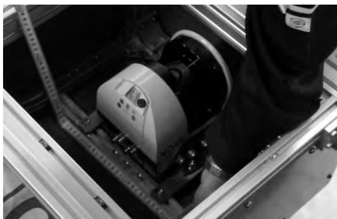
Figure 12.13 Attach the Laser scanner to rear platform
