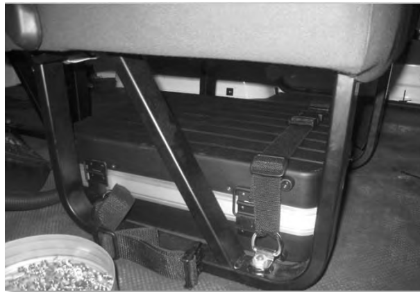
Figure 12.23 Fixing the tool box on the floors
