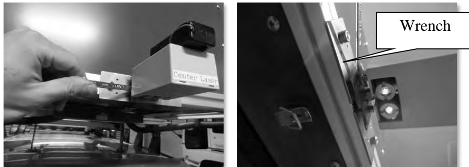
Figure 13.30 Adjusting Parts for Roll Angle
