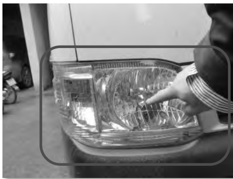
Figure 14.16 Check the lighting of the light. Check the damage of the cover of the light
