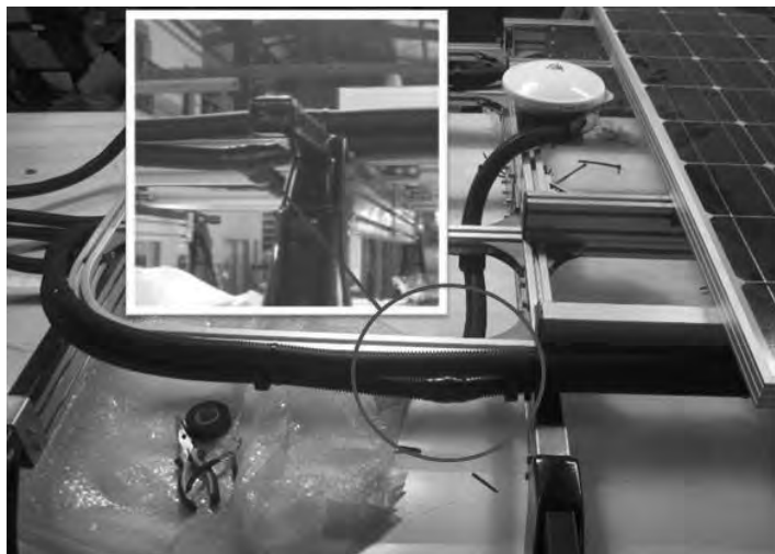
Figure 12.26 Connecting and fixing the cable of GPS
