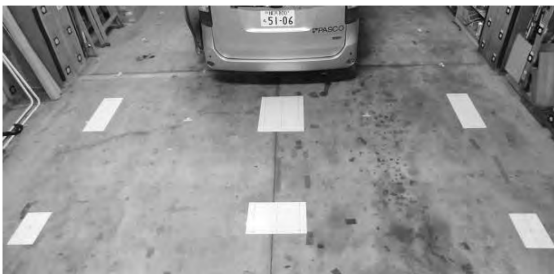
Figure 13.12 Installed Calibration Boards
