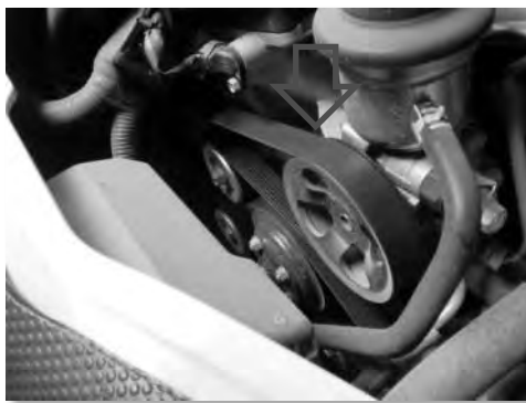
Figure 14.7 Check the fan belt( Tension, Damage)
