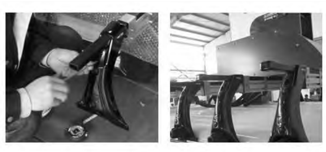
Figure 12.11 Attach the legs to front platform
