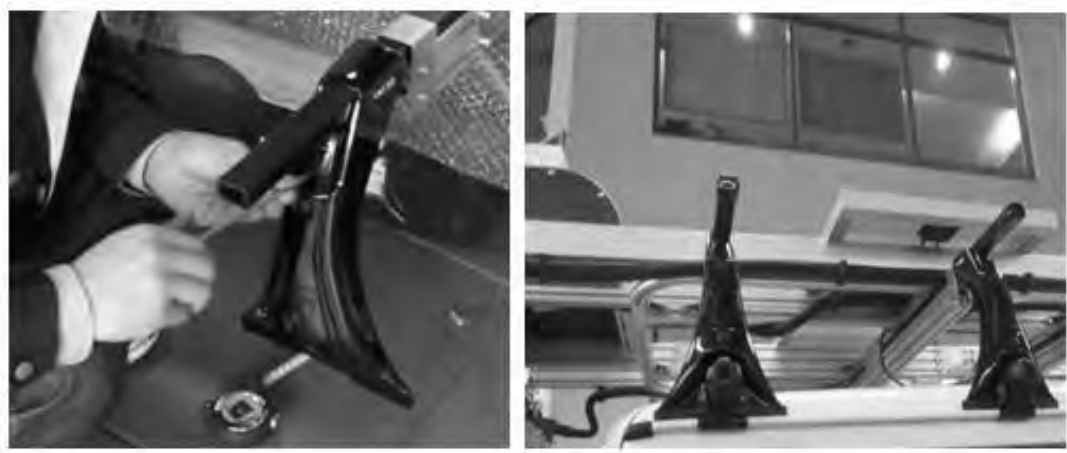
Figure 12.15 Attach the legs to rear platform
