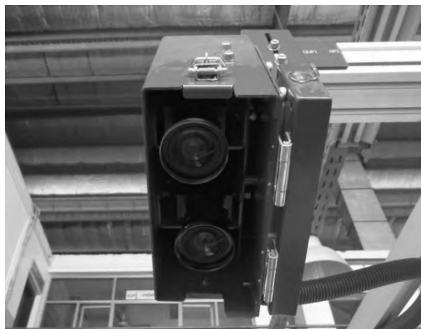
Figure 12.21 Attach cameras for road image to the rear platform
